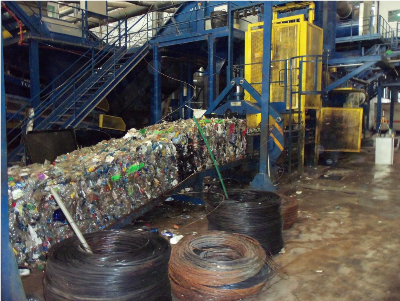
PACKAGING OF BYPRODUCTS IN A PRESS
